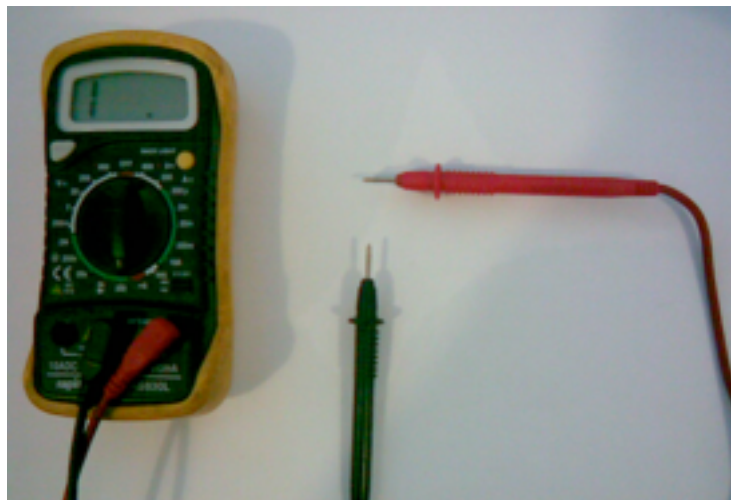
Figure 8 - an Ohm meter measuring an open circuit
