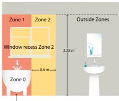
The space under the bath is: Zone 1 if accessible without the use of a tool outside the zones if accessible only with the use of a tool
