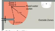
S = thickness of partition Y = radial distance from the fixed water outlet to the inner corner of the partition
